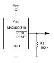
Figure 3. Ensuring RESET Valid to V<sub>CC</sub> = 0 V
