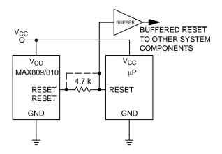
Figure 4. Interfacing to Bidirectional Reset I/O
