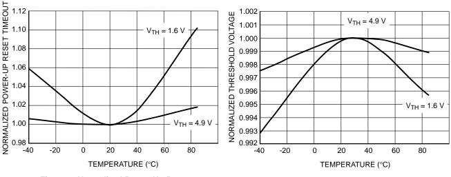
Figure 7. Normalized Power-Up Reset vs. Temperature
