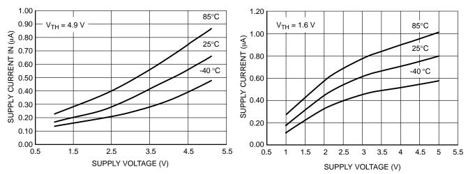
Figure 5. Supply Current vs. Supply Voltage
