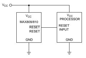
Figure 1. Typical Application Diagram
