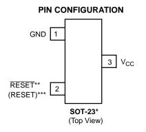
NOTE: \*SOT-23 is equivalent to JEDEC (TO-236) \*\*RESET is for MAX809 \*\*\*RESET is for MAX810
